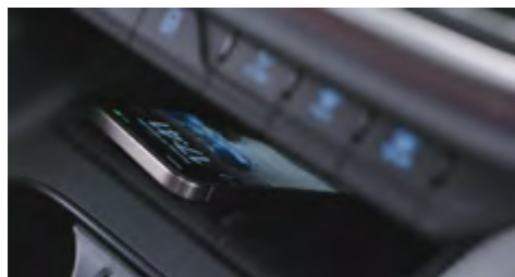
Wireless charging with cooling function
