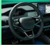
3-spoke leather heated sports multi-function steering wheel with paddles for recuperation level selection
