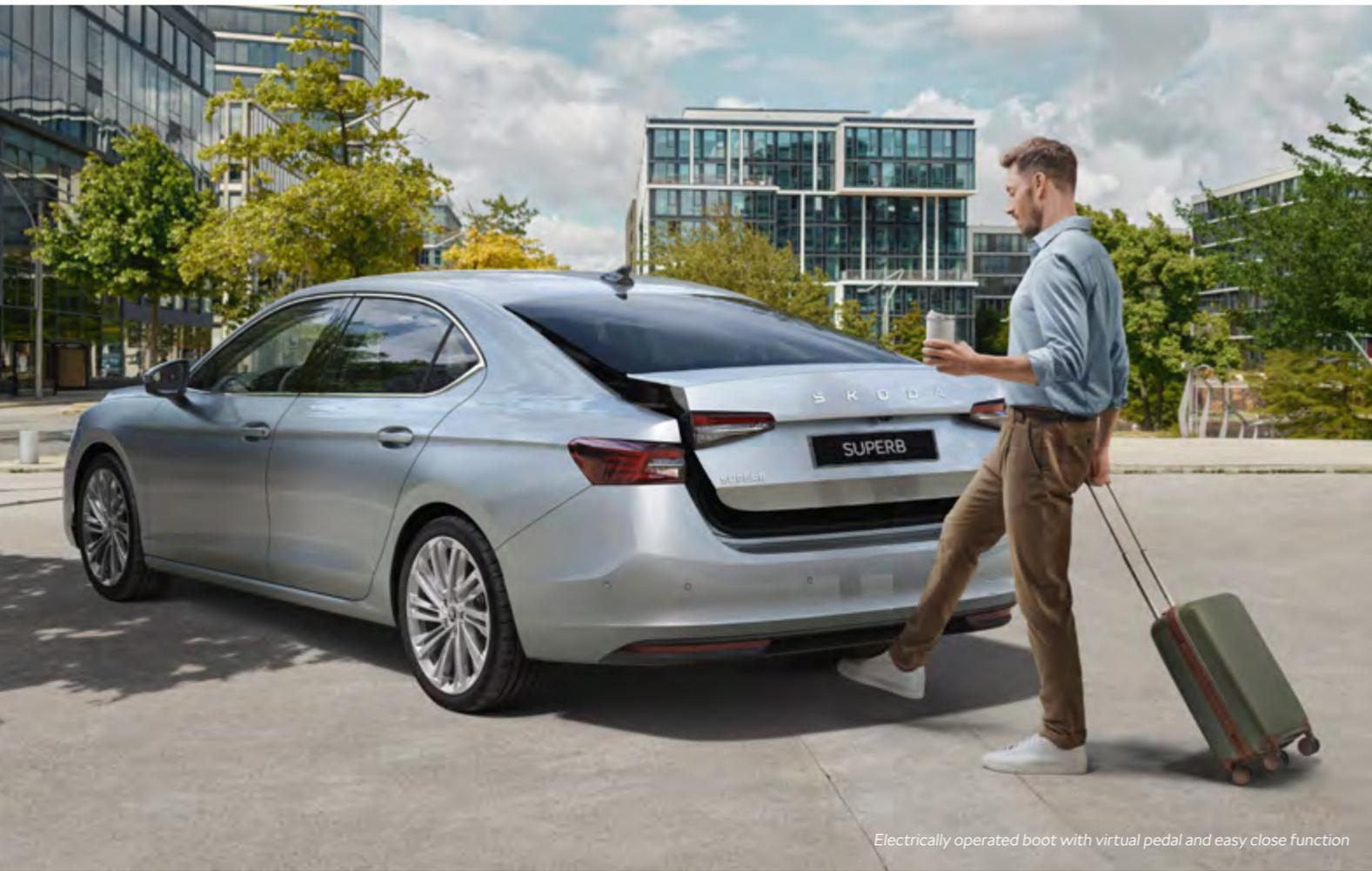
Electrically operated boot with virtual pedal and easy close function
