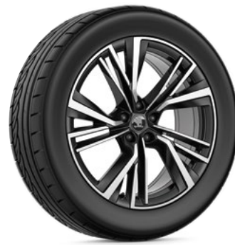
Neptune light-alloy wheel Colour: black metallic, brushed › Front: 8.0J × 20" ET 45 for 235/50 tyre › Rear: 8.0J × 20" ET 45 for 235/50 tyre** (5LA 071 490P FL8/5LG 071 490P FL8)* › Rear: 9.0J × 20" ET 42 for 255/45 tyre*** (5LA 071 490Q FL8/5LG 071 490Q FL8)* Škoda Genuine Accessories
