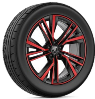
Neptune light-alloy wheel Colour: black metallic and red › Front: 8.0J × 20" ET 45 for 235/50 tyre › Rear: 8.0J × 20" ET 45 for 235/50 tyre** (5LA 071 490T CZX/5LG 071 490T CZX)* › Rear: 9.0J × 20" ET 42 for 255/45 tyre*** (5LA 071 490AA CZX/5LG 071 490AA CZX)* Škoda Genuine Accessories
