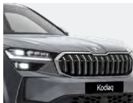
Full matrix LED headlights and front grille with horizontal light strip
