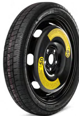
18" spare wheel – space saver 3.5J × 18" ET25.5 125/70 R18 5E3 601 011B
