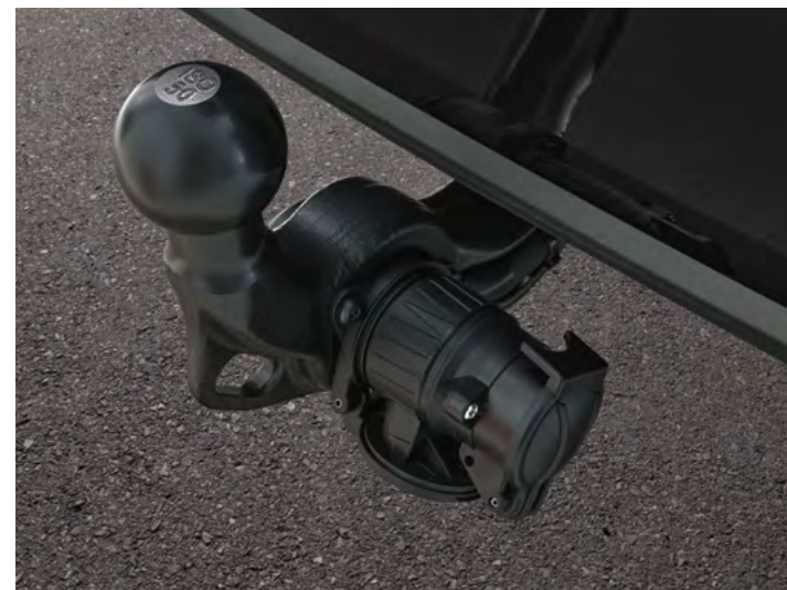
Towbar adapter – from 13-pin to 7-pin socket*
