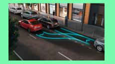
This function removes the stress of bay and parallel parking by identifying if the parking spot is big enough before automatically steering into the space.
